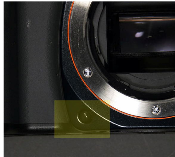
Figure 4-14: Depth of Field preview button (highlighted in yellow).
