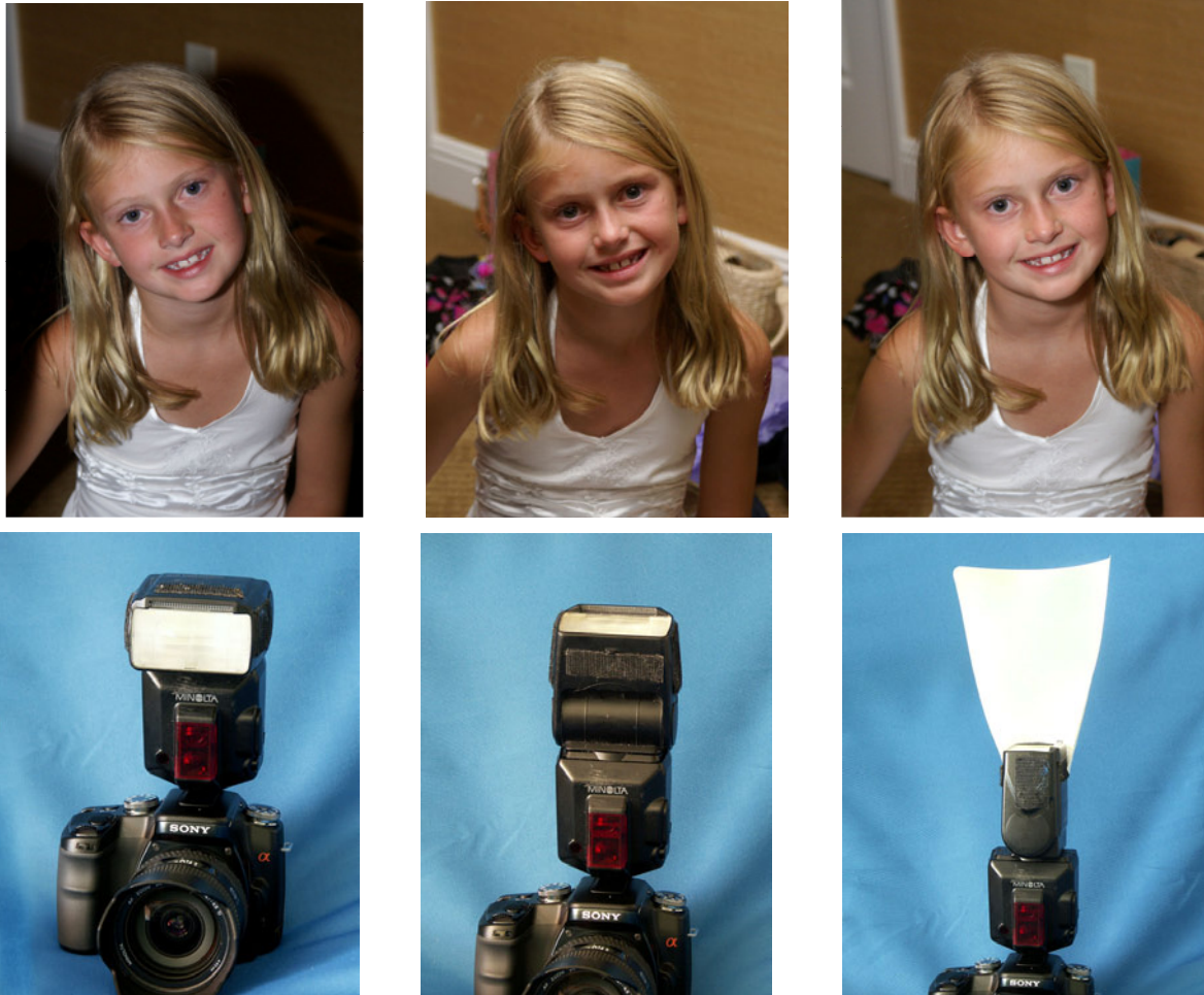
Figure 7-11: Examples of Straight on-camera flash (Yuk!) vs. ceiling bounce. The third picture uses an easy-to-make light modifier which takes some of the light destined for the ceiling and converts it into a soft, pleasing subject light. What a difference!
