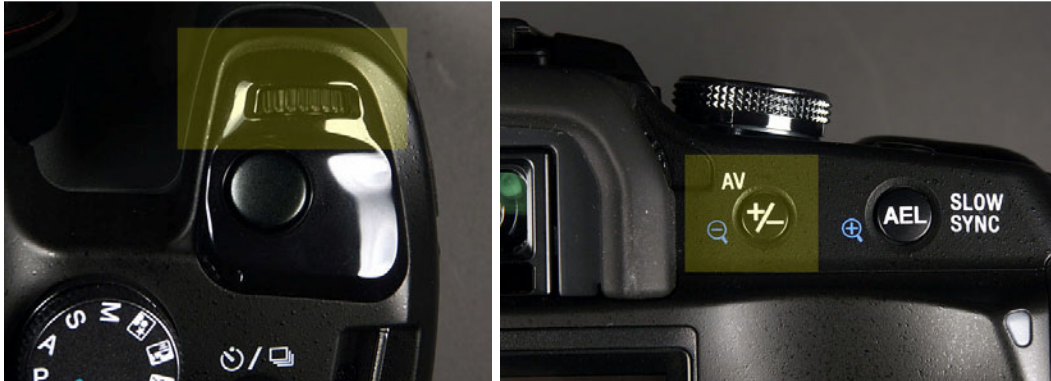
Figure 4-18: When in Manual exposure mode, you can change the shutter speed by rotating the front control wheel. To change the f/stop, hold down the exposure compensation button (labeled “+/-”; right) while rotating the front control wheel.
