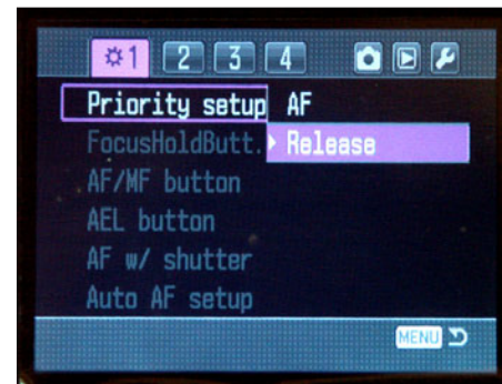
Figure 2-14: Release Priority tells the camera to take the picture when YOU want, not when the camera thinks it should.
