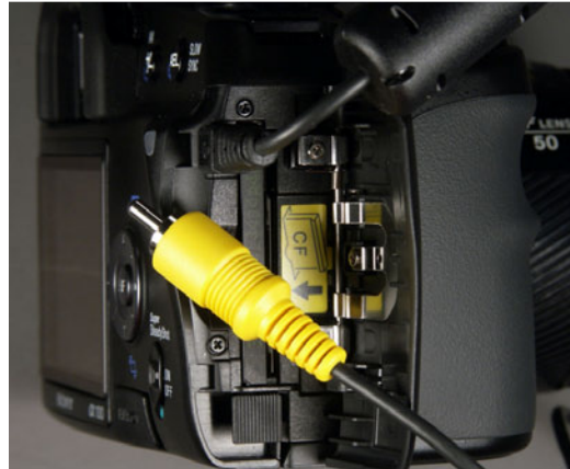
Figure 3-8: Hooking up the camera to a TV via the supplied video cable. (The cable connector is inside the memory card door.)
