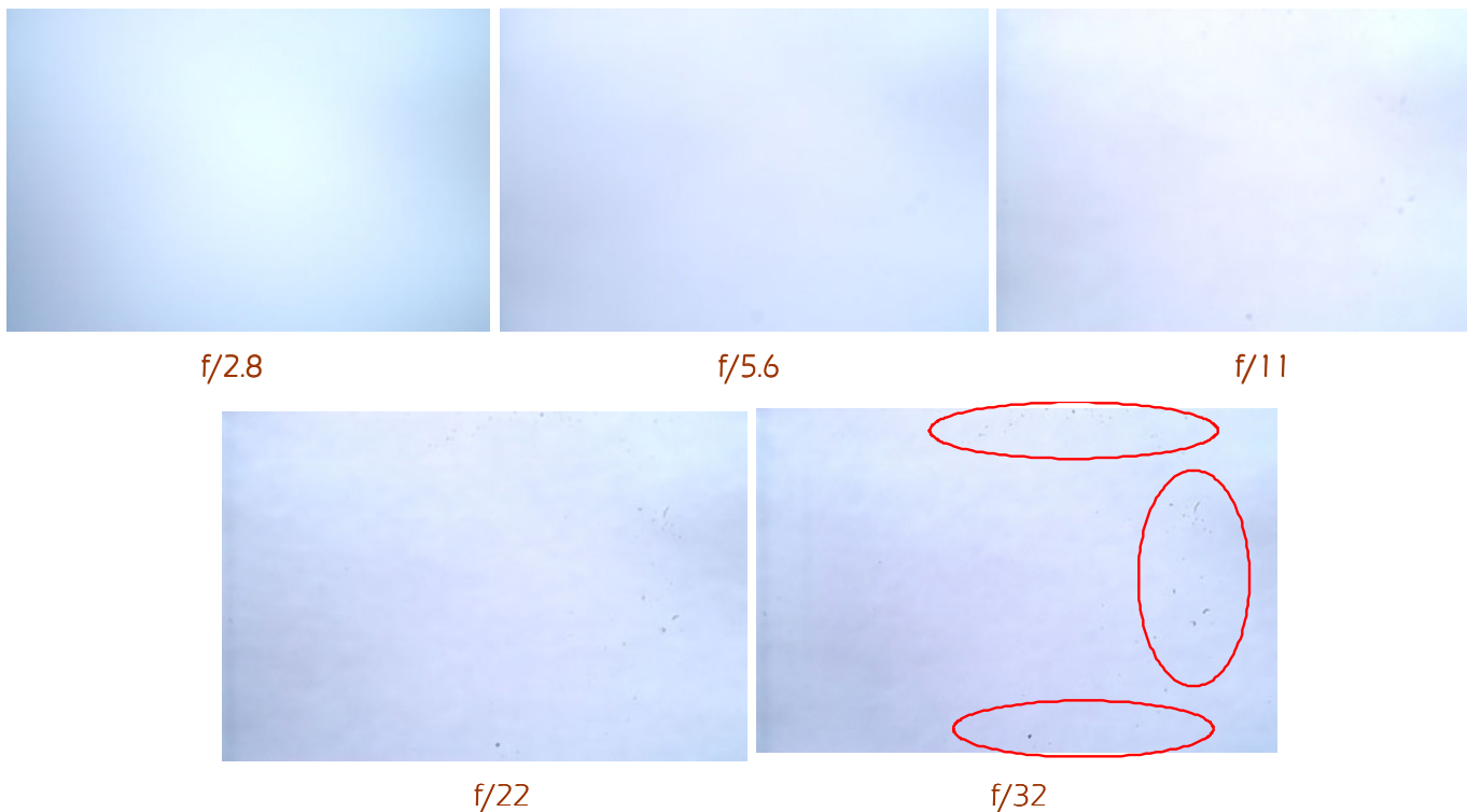
Figure 8-6: Dust doesn't usually show up in your images unless you're shooting with small f/stops, like f/32. Above are five pictures (with the contrast enhanced so that the dust appears more visible); notice that at f/2.8 it doesn't appear at all, but as you make the lens opening smaller the dust begins to appear more blatant. You should check for dust at least once a month and remove it immediately when found; for it becomes more difficult to remove the longer it is there.
