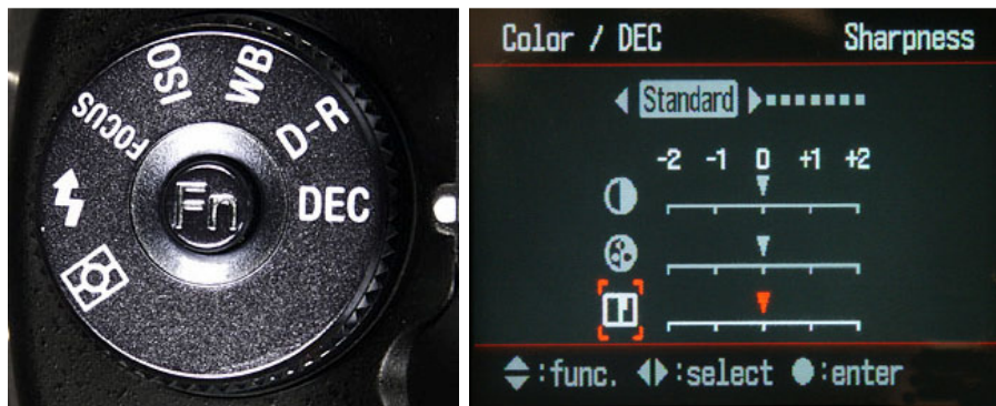
Figure 5-40 The Digital Effects screens control color space, contrast, sharpness, and color intensity (saturation).
