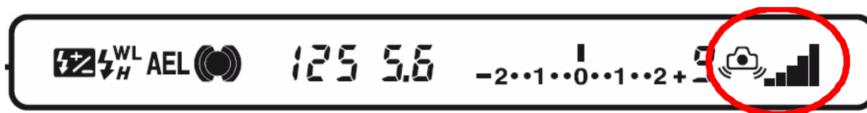
Figure 5-9: The Super SteadyShot scale in the lower-right-hand corner of the viewfinder shows you how shaky your hands are, and therefore how hard the system will have to work. For best results, wait a few moments until the number of bars is reduced (showing how the system adapts) before shooting.
