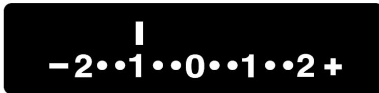
Figure 4-16: The viewfinder scale in manual mode. Here, the camera's exposure meter is telling you “I think you're providing the sensor with one stop less light than you should for an average scene!” Fortunately, in this case you wanted to underexpose by one stop, so you can safely shoot away after receiving (and then ignoring) this feedback!
