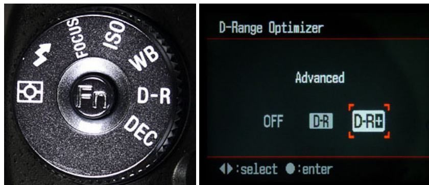
Figure 5-38: Invoking one of two Dynamic Range Optimization (DRO) functions.
