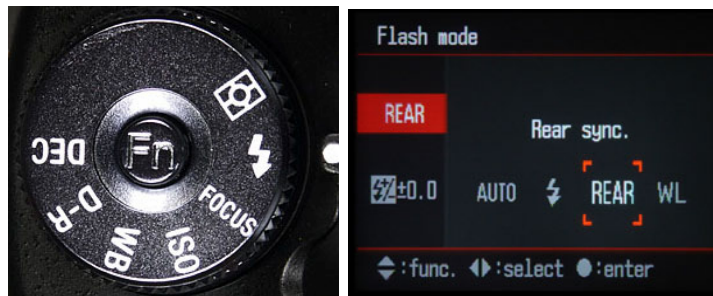
Figure 5-25: Invoking the Rear Sync function.
