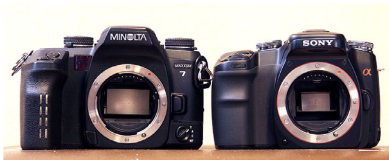
Figure 1-6: The camera on the left is the Minolta 7 film camera, whereas the camera on the right is the Alpha 100. Notice that the mirror on the film camera is larger than on the digital; so too is the sensor smaller behind it (which you can’t see in this picture). This is the reason that all lenses have a 1.5x “Crop factor”. The text has more info.
