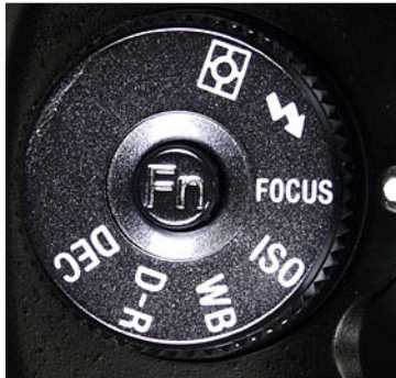
Figure 2-11: To change the focus point, rotate the function dial until the word "FOCUS" aligns with the white dot, and then press the center button.
