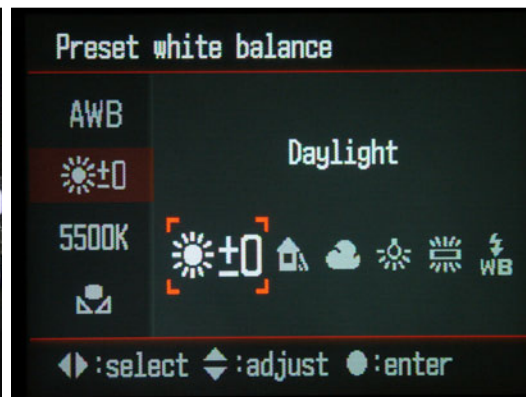
Figure 5-11: The Pre-set White Balance Setting and its associated screen.
