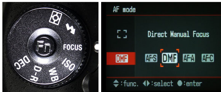
Figure 5-3: How to invoke Direct Manual Focus mode.
