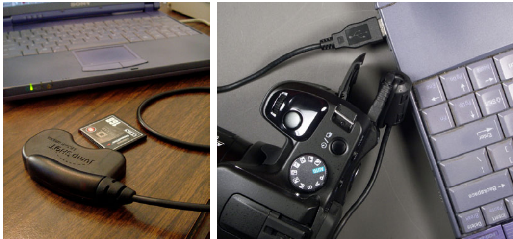
Figure 3-9: You can plug the memory card into a computer with suitable hardware to read it, or you can hook up your camera directly to the computer (via the supplied cable) and have it appear to the computer as an external disk drive.
