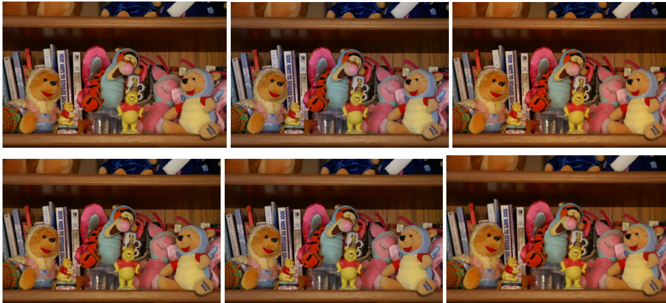
Figure 5-32: White Balance Bracketing Examples. Top row is “Low bracketing” (Normal → blueish → yellowish]; and the bottom row is “High Bracketing”. The difference is “High bracketing” will shift the color twice as much in either direction.
